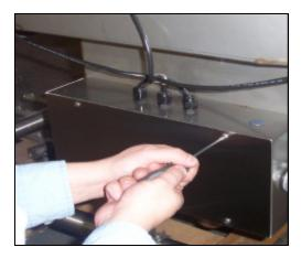
Removing the heater box cover
